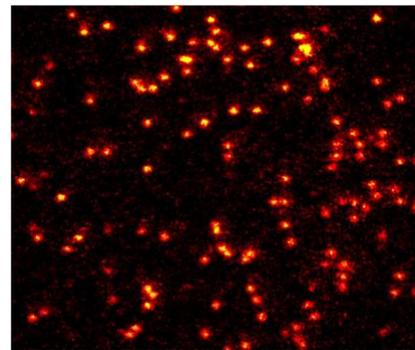
Potassium 40 atoms pinned in an optical lattice and exposed to cooling laser beams. The atoms absorb and re-emit photons which are collected via a high resolution objective. Each bright spot signals the presence of an atom with a fidelity > 99.6%. This method has also been demonstrated for <sup>6</sup>Li. *Courtesy of M. Zwierlein MIT*
