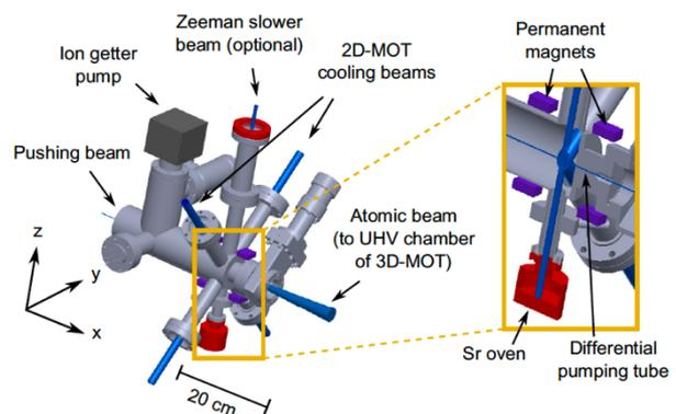
*Experimental setup of a 2D MOT of Sr atoms, taken from I. Nosske & al., Phys. Rev. A 96, 053415 (2017).*
