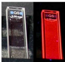
Electron microscopy image of a YVO 4 :Eu nanocrystal and photographs of a colloidal suspension in white and UV light showing the red luminescence characteristic of Europium Eu 3+ .
