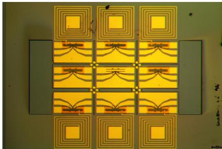
GHz resonators made of topological edge states
