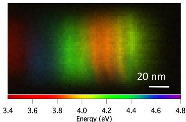
An alternative, largely pioneered in our group, is to use electron-based microscopies and spectroscopies. Indeed, electron energy loss spectroscopy (EELS) and cathodoluminescence have been very successful for the deep sub-wavelength investigation of several nanooptical objects and excitations, such as plasmons, quantum wells and single photon emitters.
