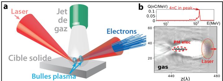
a- Hybrid target principle: solid + gas target.
