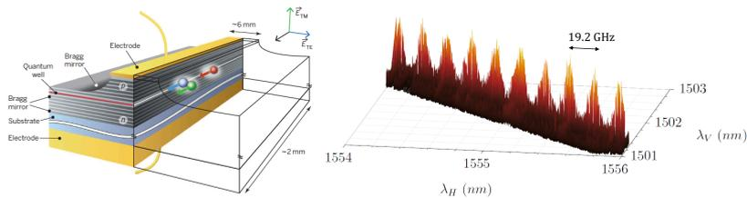
*Left: sketch of an electrically driven photon pair source working @ room T; Right: measurement by stimulated emission tomography of the biphoton frequency comb emitted by our devices*
