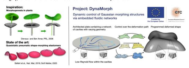
In this internship, you will develop 3D-printed soft architected structures containing a network of interconnected cavities. By controlling the flow and the pressure distribution within the soft architected structure, the aim will be to characterize and then rationalize the fluid structure interaction at play to program the shape changes in space and time.
