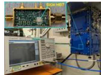
Insert : BiCMOS chip packaged to enable characterization and making a functional amplifier for quantum bits experiments. Measurements with a vector network analyzer will be performed in a cryostat (blue cubes).
